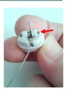
Place the female finger middle frame on the spring axle, making sure the end of the spring and the finger cable remain inside the frame.
