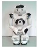
Press the chest button for 3 seconds until the robot says "GNUK GNUK".
